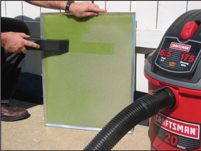
*Vacuum method – A shop vacuum can be used to remove accumulated dust and debris.*
