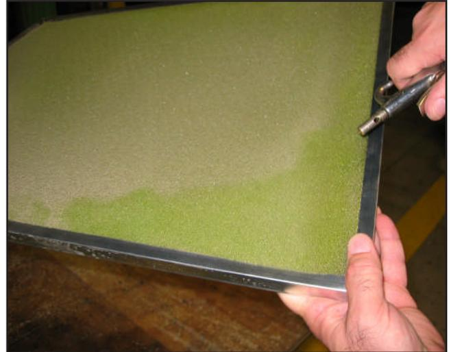
*Compressed air method – Use compressed air to blow out dust and debris in the opposite direction of the air flow on the charger.*
