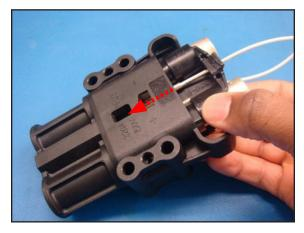
6. Confirm the contacts are inserted in the proper locations as shown.
