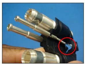
5. Re-insert the contacts assembly into the main connector housing and snap it into position to lock it into place.
