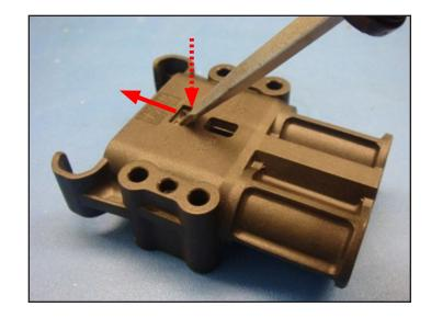
2. Remove the contacts assembly from the main connector housing.
