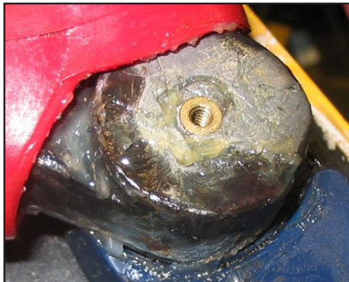
Knurled Brass Insert Installation
