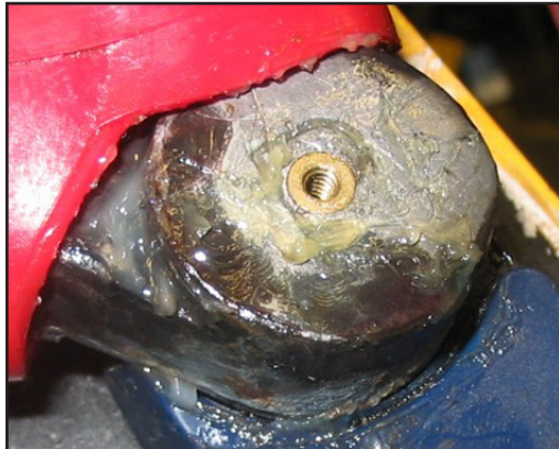
Knurled Brass Insert Installation
