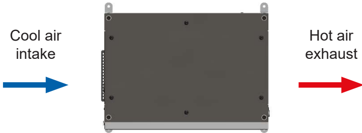
Figure 1 Side-to-Side Airflow Design, Top View
