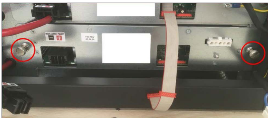
Figure 31 Replacement Power Module Insertion
