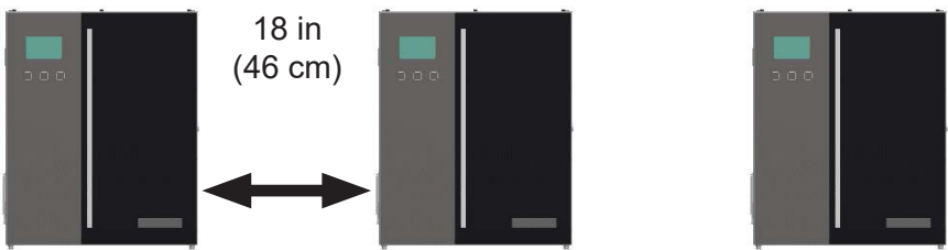
Figure 2 Standard Side-to-Side Charger Spacing
