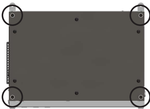
Figure 5 Attaching Points for M8 Lifting Eyebolts, Top Panel View
