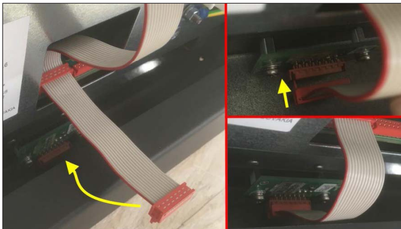
Figure 35 Flat Cable Connection to the Termination Block
