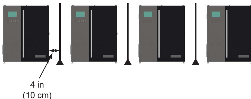
Figure 3 Side-to-Side Charger Spacing with Dividers
