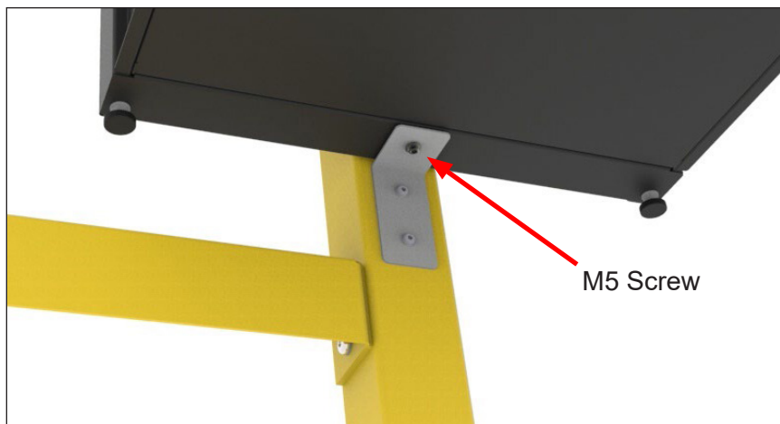
Figure 13 Bottom Bracket Mounted to the Charger and Floor Stand with a Tightening Torque of 52.22 in-lbs (5.9 Nm)
