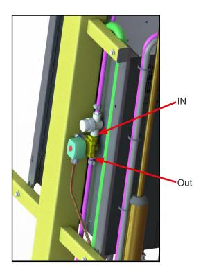
11. Attach the watering hose to the charger output connector with a cable tie as shown below, then secure the hose to the output cable with a cable tie every two inches. When finished, cut off any excess hose, slip the hose over the barbed fitting on the valve, and secure it with a metal hose clamp.
