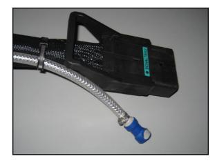
12. Use cable ties to secure all the loose hoses to available location on the complete assembly as shown below.
