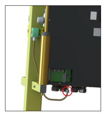
9. Connect one red wire to the negative (-) and another red wire to the positive (+) electrical connections, then connect the green wire to the earth/ground connection as shown bellow.
