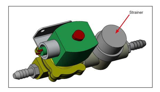
7. Mount the valve to the left side of the pedestal using two 1/4-20 x 1/2 flanged bolts (P/N # 01860).
