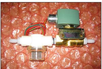
6. Confirm it is correctly positioned to the strainer as shown below.
