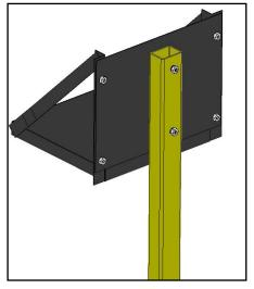
3. Mount the extension bracket (P/N # 25394) to the pedestal with two 5/16-18x3/4 flange head cap screws (P/N # 24759) from front of extension bracket, two 5/16-18 Hex nuts (P/N # 06897), and two flat washers (P/N # 05241) to the rear side of pedestal.
