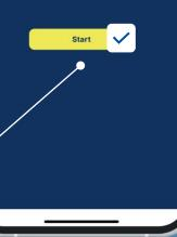
After you have started the charging station successfully, you may hear a cracking sound from the station to confirm the charging start. The LED color changes also.
